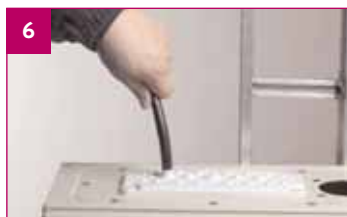
6 Pull the cable or tube back approximately 20 mm to lock it.
