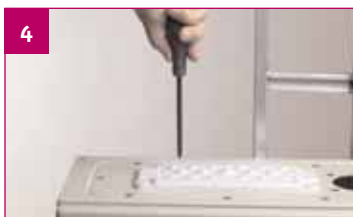
4 Make a small hole in the membrane.
