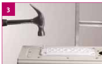
3 Drive the core of the rivet with a hammer to lock in place, or tighten fixing screws.
